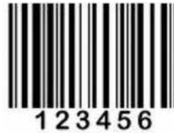
FIG. 6: Conventional barcode storing the number 123456
